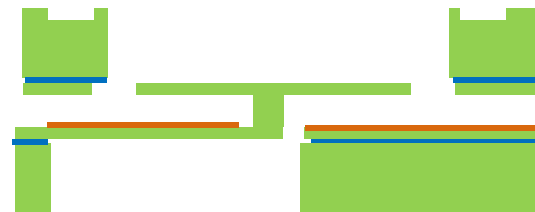
(3-f) Annealing (HfO 2 crystallization)
