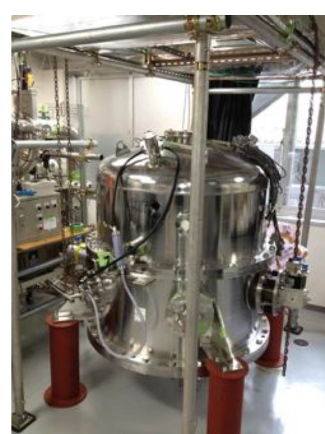
Optics of GIMMICS. The diameter of the base plate is 800mm.
