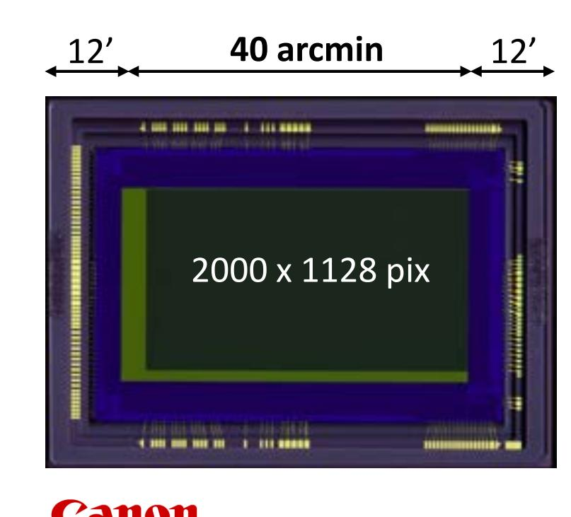
35 mm full HD CMOS sensor developed by Canon and U-Tokyo based on products for commercial use.
