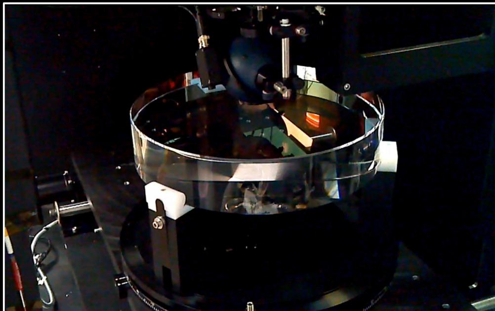
Beamsplitter(370mm dia) during coating characterization
