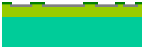
(a) Photolithography, SiN etching
