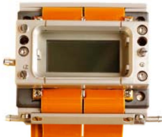
Figure 11: Fully packaged and wire-bonded SLM assembly.
