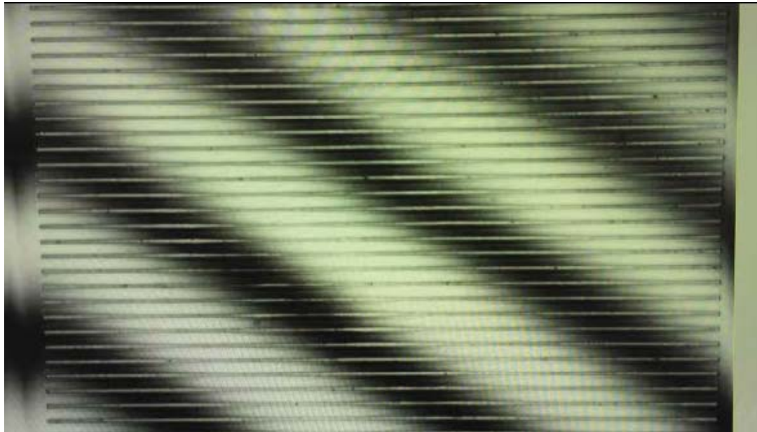
Operation of addressed ribbons of grating
