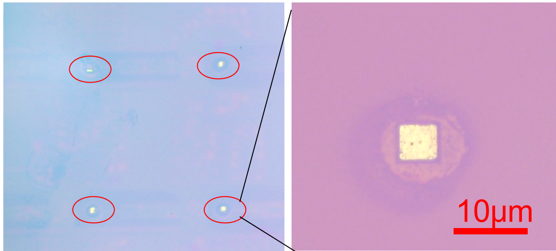
The optical micrograph of the mirror membrane with the square Au-Si reaction area
