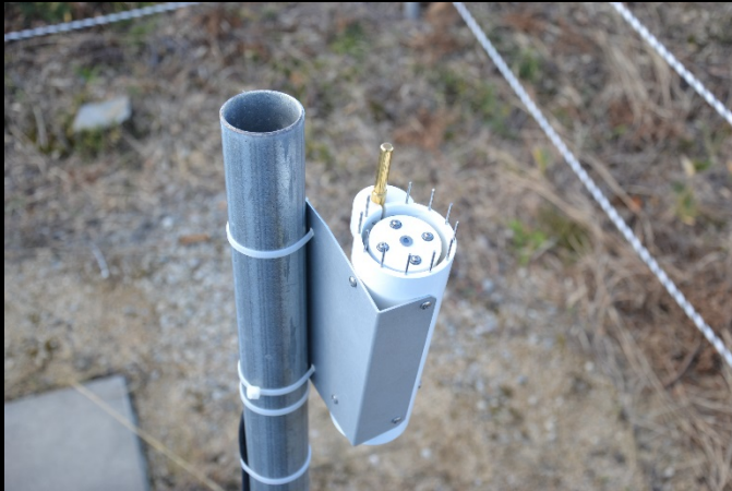
Boltwood Cloud Sensor II from Cyanogen Imaging measures the sky screen temperature.
