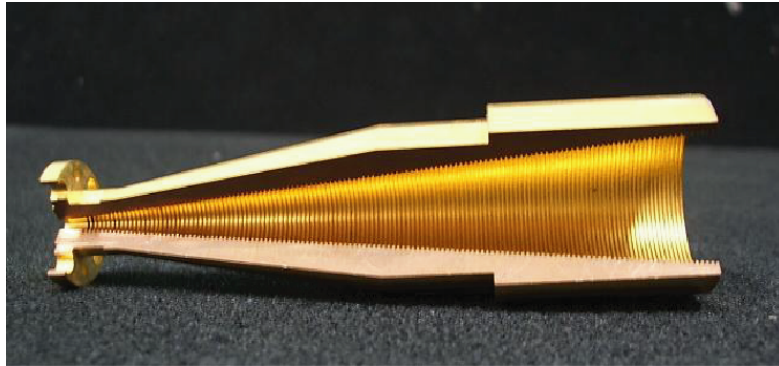
Cross-sectional view of the machined corrugated horn.
