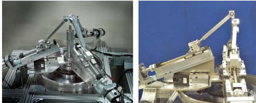
Movable-Die Drive Mechanism Using 3-RPSR Parallel Mechanism with High Orientation Capability
