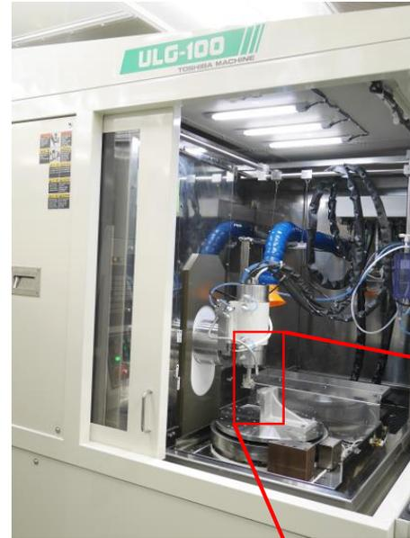
5-Axis Ultraprecision Machine (ULG-100D, Toshiba Machine)
