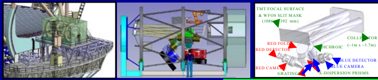
WFOS: Wide Field Optical Spectrograph. The first generation instrument for TMT. R= 500~5,000 (150~7.500 goal) @0.75" slit
