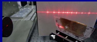
Diffraction beam of VB grating
