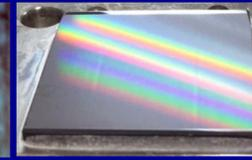
Si grism:  $\alpha = 4.2^\circ, \Lambda = 17.09 \mu\text{m}$ .
